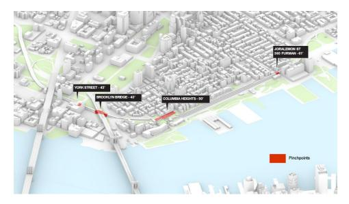
In the case of Columbia Heights, the roadway is itself a bridge structure over the BQE. A portion of Harry Chapin Playground is also on top of the bridge. This portion of the BQE, including the
