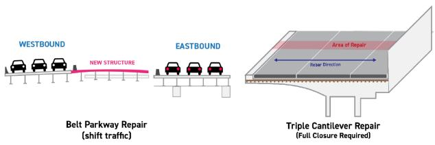
Comparison of Tradition Bridge Repair vs Cantilever Repair
