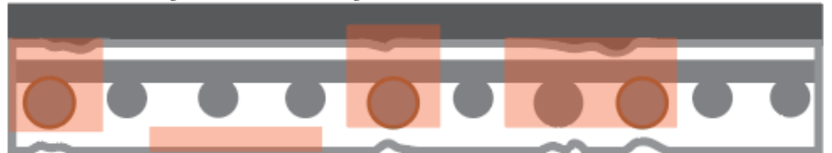
Partial-Depth Deck Replacement
