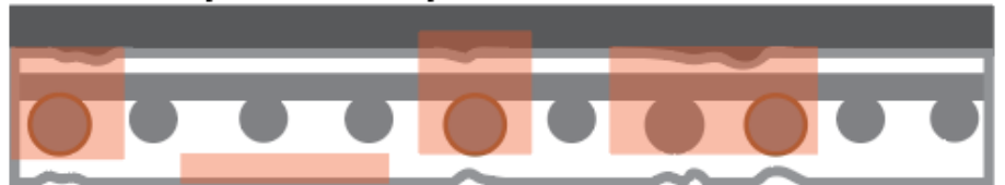
Partial-Depth Deck Replacement
