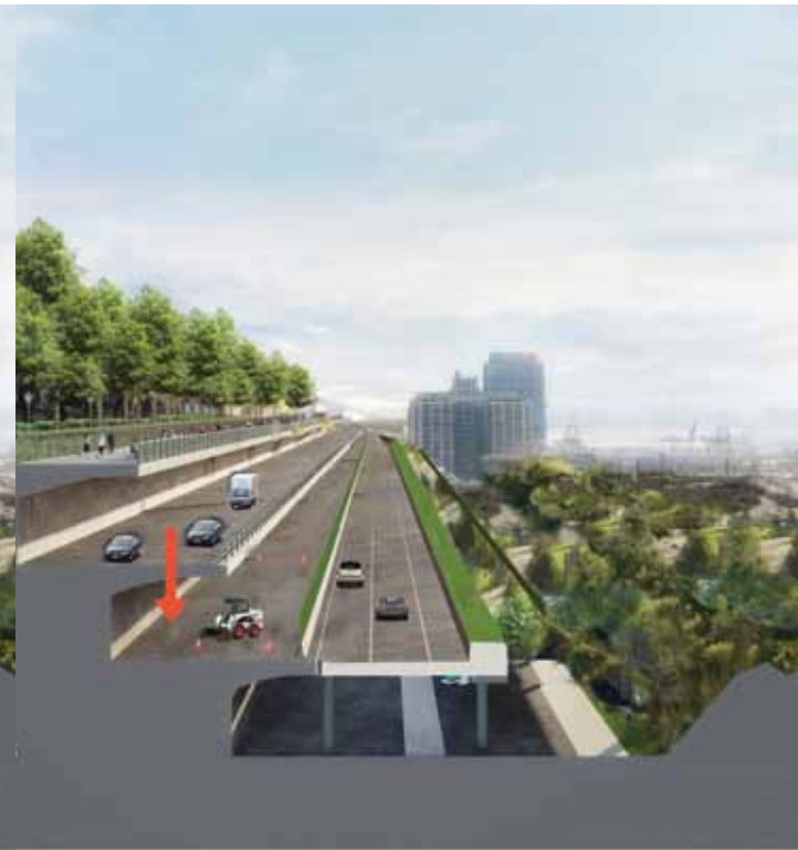
Phase 3: Transfer traffic to lower deck
