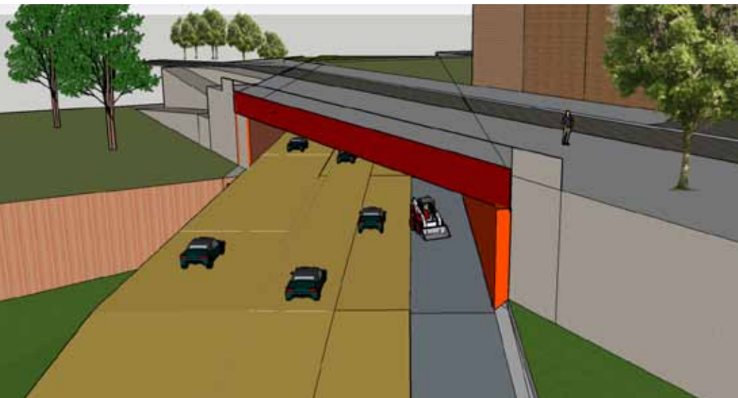
7. Columbia Heights Bridge: New beam set at higher elevation
